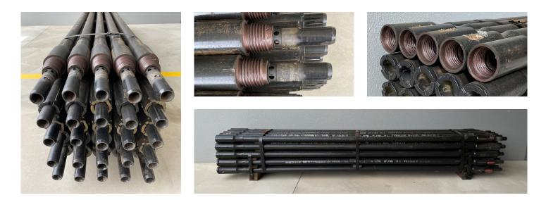
Premier horizontal directional drill rods are a premium manufactured product. Starting with 4137H extra wearresistant bar stock and heat treat the tool joints to oilfield API S135 specifications for ultimate fatigue resistance.
