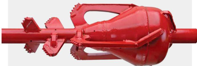
Heavy duty blades with carbide teeth for aggressive cutting action.
